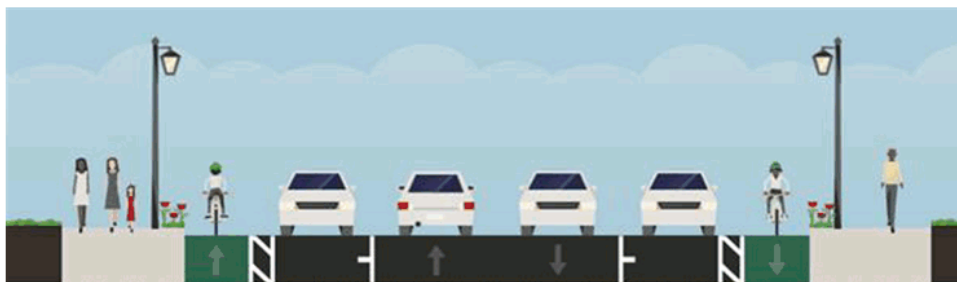
Figure 47 - Alternate cross section of Vincent Street (slow speed mixed traffic).
