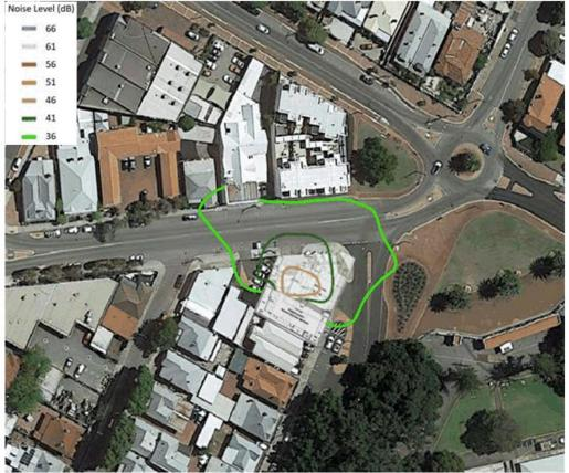
Figure 3 – Forecast L<sub>A10</sub> night-time noise contours @ 4.5m above ground (Residential Assigned Level = 41 dB)
