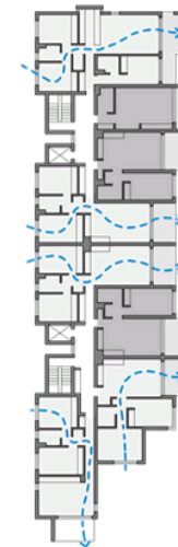
Figure 4.2a Five out of a total of eight apartments in the above example can achieve natural cross ventilation with dual aspects / corner layout. The remaining three single aspect apartments cannot achieve cross ventilation.
