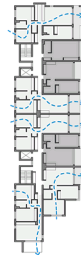
Figure 4.2a Five out of a total of eight apartments in the above example can achieve natural cross ventilation with dual aspects / corner layout. The remaining three single aspect apartments cannot achieve cross ventilation.
