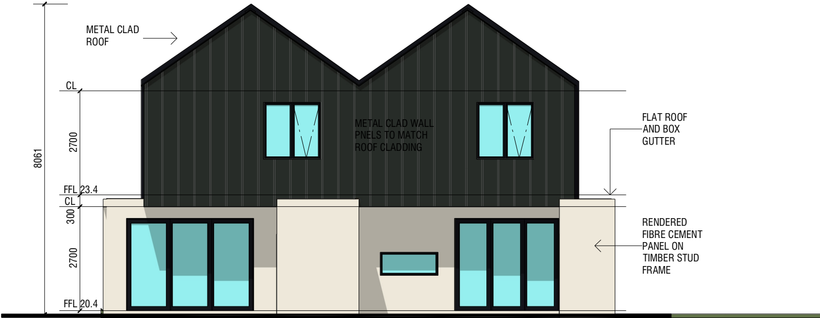
ELEVATION 03 (rear units 5,6) SCALE 1:100
