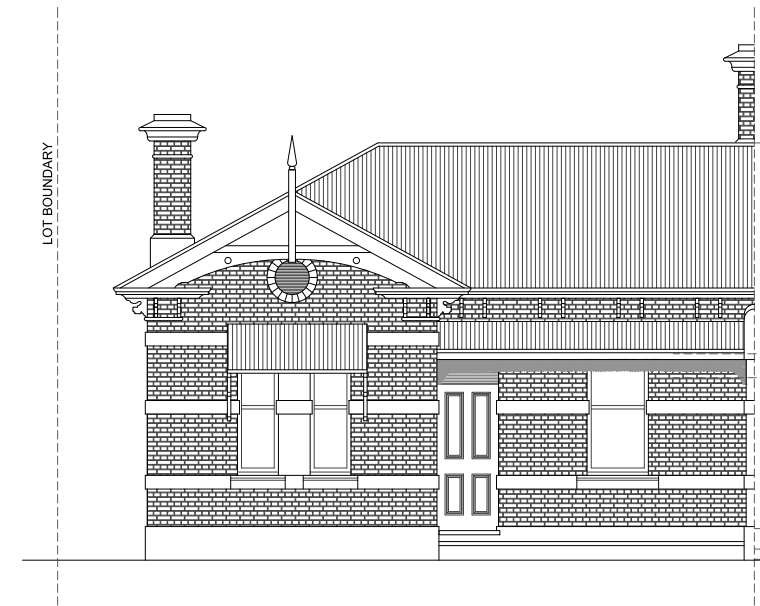
EXISTING WEST ELEVATION
