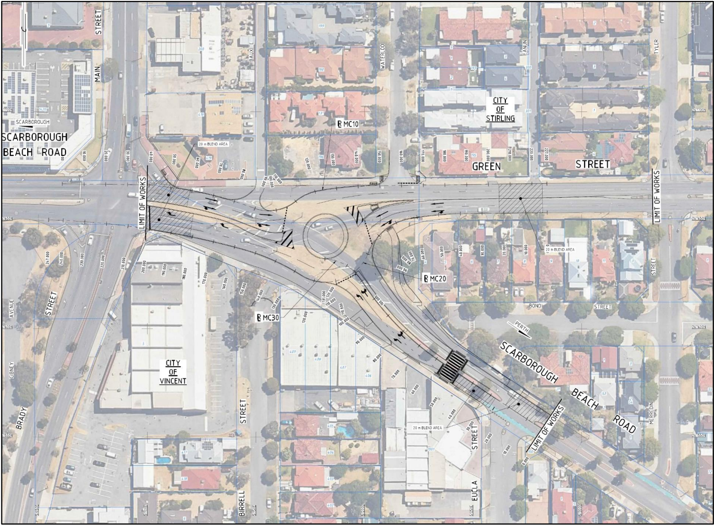
Figure 2 - Detailed Design Plan of Proposed Intersection Modifications
