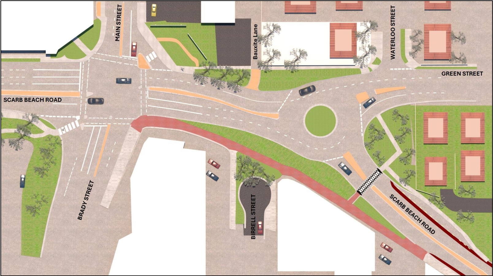
Figure 1 - Concept Design Plan of Proposed Intersection Modifications
