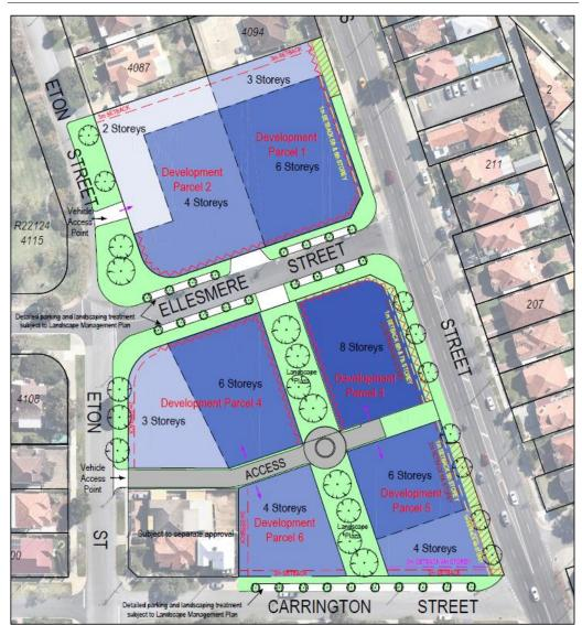
Figure 3.1: Concept layout plan
