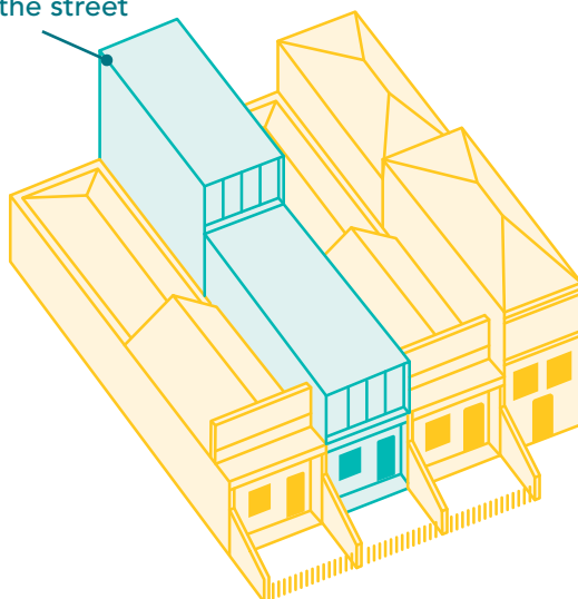
Figure 5: Siting of upper floor additions
