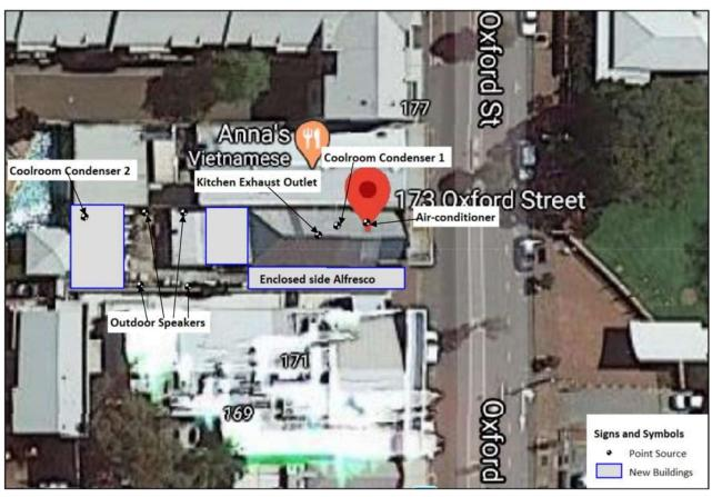
Figure 7: Locations of outdoor noise sources assumed in the acoustic model.
