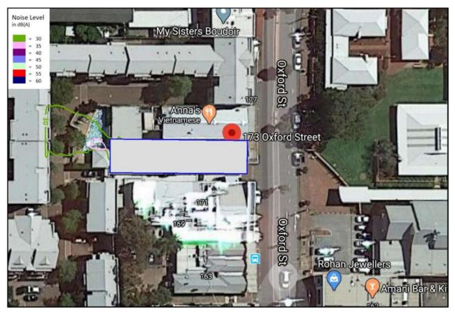
Figure 9: Worst-case night-time noise contours for scenario 1A at 1.5m above the ground.
