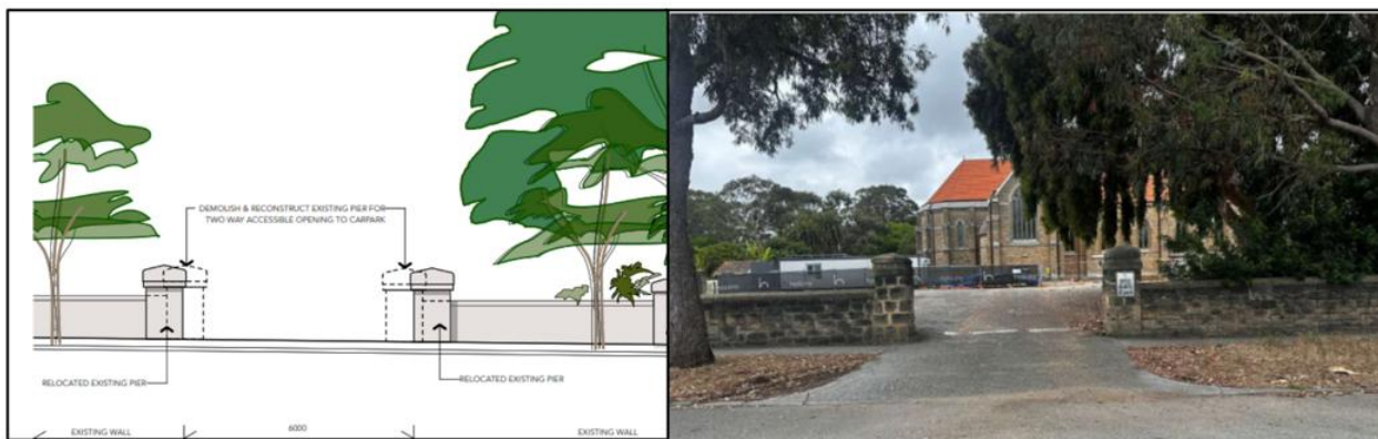
Figure 2: Proposed increase to the existing driveway on Alfonso Street to allow for two-way access and reconstruct two limestone piers (left) and existing limestone wall and entry point (right)
